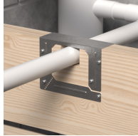
Reinforces solid joists where notches have been cut into them to allow services to pass through.
