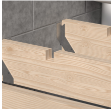
Step 1: Carefully mark and cut out the notch in the joist.
