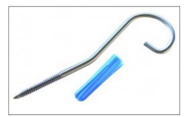
Screw in wall starter with nylon wall plug, WST provides lateral stability to brickwork or blockwork walls. Can be installed horizontally or at a 30° angle to the mortar joint.
